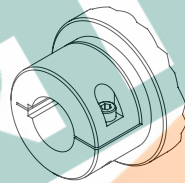
Type B1 Single split clamp hub with H7 bore and keyway.
